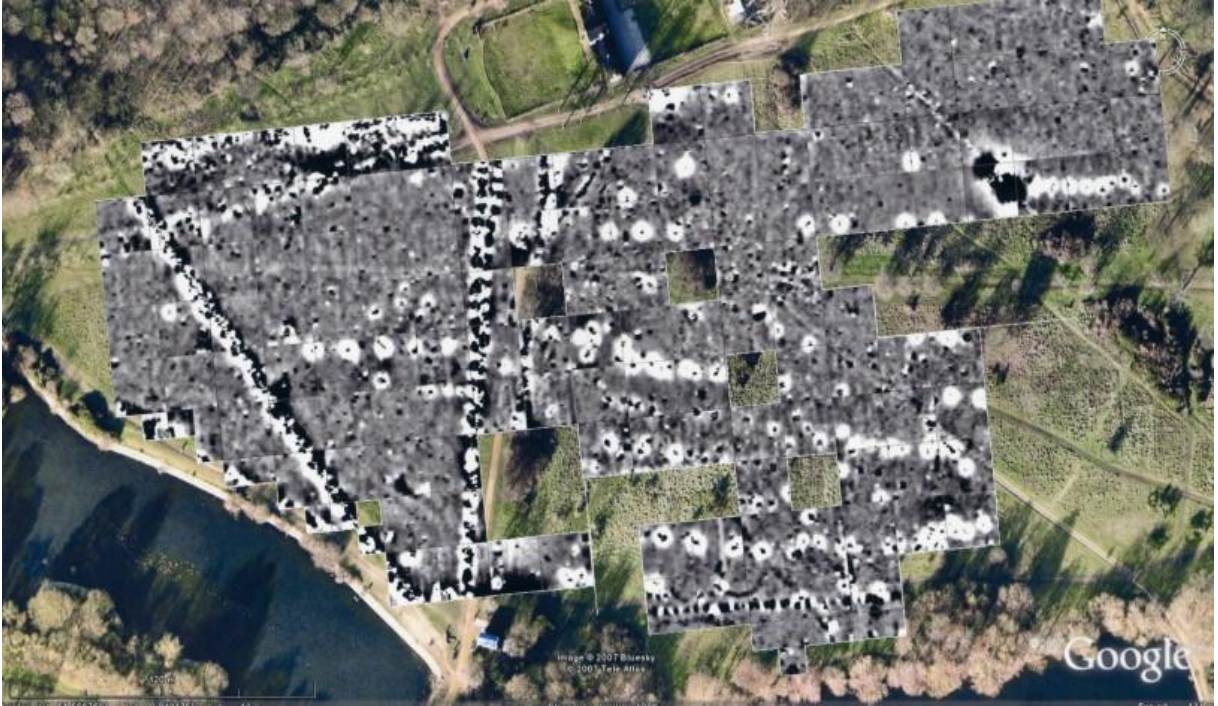
Figure 3. Magnetometer survey 1 x 0.25m, 20m transects, SN zigzag progressing E, -2 to +3nT, dark positive (processed by Dr Tim Dennis, University of Essex)
