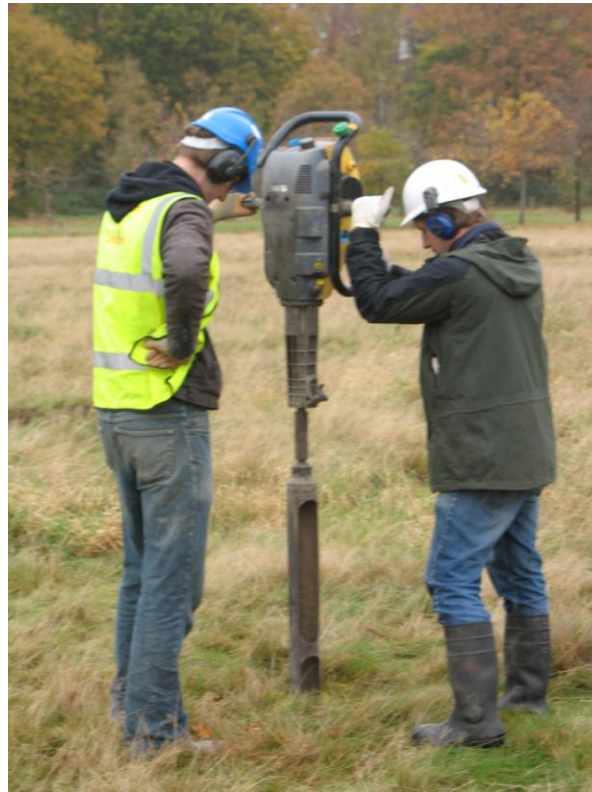
Figure 14. The power auger in use.
