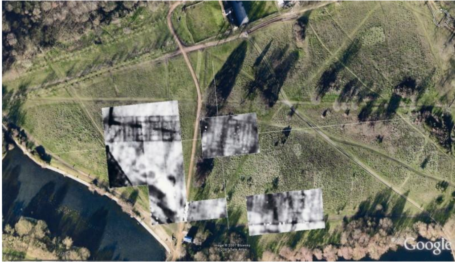
Figure 12. Resistivity survey 1 x 1m, 20m transects, twin probe configuration, 0.5m probe spacing, SN zigzag progressing E, ohms range 100 to 1000 Dark low resistance
